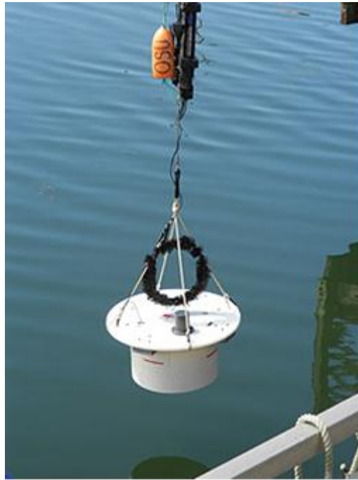
Gambar 13. Lowering the Benthic Microbial Fuel Cell (BMFC) into the water Image: Oregon State University
